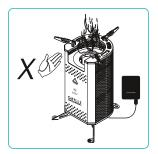
Do not touch the top parts of the stove when cooking. Be careful the of high temperature.
