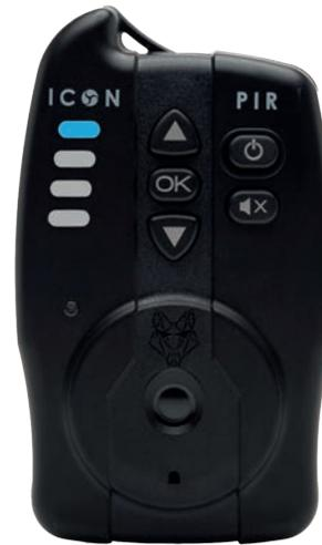
From idle, Press OK to enter channel browsing mode. Use ▲ and ▼ to select an unpaired channel, indicated by a fast blinking red indicator. Press and hold
