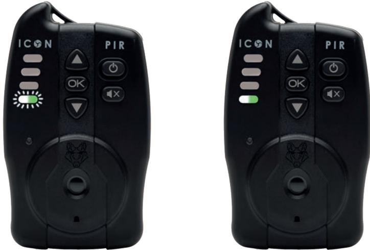
All paired devices will be muted/unmuted. The corresponding channel LED will flash white/green while the communication is in progress.
