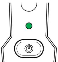
After power on the PIR will start an arming sequence, with a flashing of the LED in the selected alert colour. The flashing gets faster as the sequence completes.
