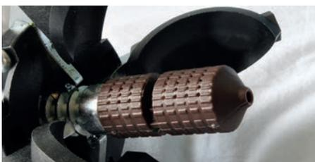
Screw Method Feeder on to Ball Maker.
