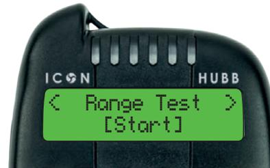
Navigate to the option 'Range Test' and use the OK button to begin the test. When a connection is established the HUBB will report the signal strength of the connected Alarm and also indicates that the LED is working.
