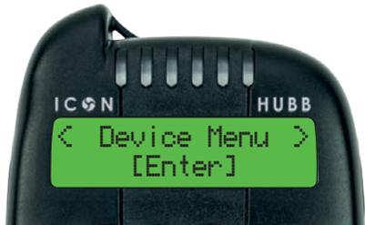
On activation of the bite Alarm the tone is replicated on the HUBB and the HUBB LED's replicate the alert colour shown on the bite Alarm. Depending on the HUBB's settings, the HUBB will also vibrate on alert.
