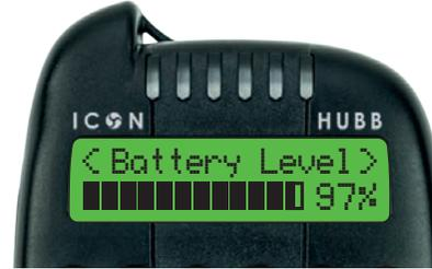
Navigate to the option 'Battery Level'. This provides a detailed measurement of the Alarms battery level.
