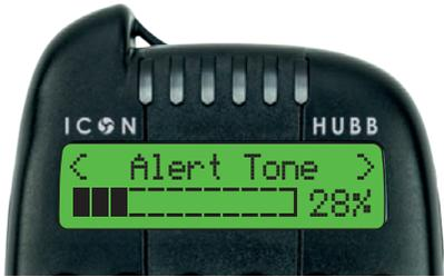
In 'Advanced Menu' go 'Alert Tone' to adjust the pitch on the Alarm and the HUBB.
