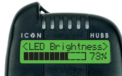
Go to **'LED Brightness'** to change the brightness of the LED's displayed on the bite Alarm.
