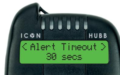
Go to **'Alert Timeout'** to adjust the time that the LED remains turned on after an alert on the bite Alarm.
