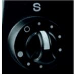
The sensitivity knob adjusts the amount of line travel before an alert is triggered. There is also an Off position to turn the Bite Alarm off. 8 Sensitivity Levels, expandable to 16 via HUBB link. 2mm, 6mm, 11mm, 17mm, 25mm, 34mm, 61mm, 101mm. \*Additional HUBB Settings 4mm, 8mm, 16mm, 20mm, 30mm, 40mm, 80mm & 100mm.
