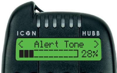
In 'Advanced Menu' go 'Alert Tone' to adjust the pitch on the Alarm and the HUBB.
