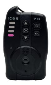
From idle, Press OK to enter channel browsing mode. The last channel to receive an alert will be selected by default, and its corresponding channel LED will pulse in the selected alert colour. If the channel is unpaired, the channel LED will fast blink red.
