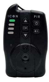
From idle, Press OK to enter channel browsing mode, double press the  $\ensuremath{\mathfrak{O}}$  power button to toggle the paired device's 'Device Option'.
