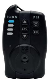
From idle, Press OK to enter channel browsing mode. Use ▲ and ▼ to select an unpaired channel, indicated by a fast blinking red indicator. Press and hold ■× to initiate pairing.
