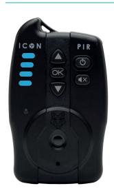
To return the PIR Sounder to factory settings, and clear all user data, power the PIR Sounder off, and then power it back on while holding the \*\* key. When all the channel LED's turn Blue, release only the \*\* key while keeping \*\* pressed. After the Blue LED's have flashed and turned Off, the PIR Sounder can be turned back on by holding \*\*U.
