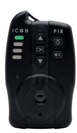
From idle, Press OK to enter channel browsing mode. Use ▲ and ▼ to select a paired channel, indicated by a pulsing indicator LED. Press and hold ◄× until indicator turns BLUE. Release then indicator will blink RED.
