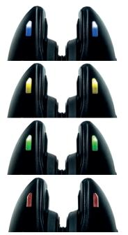
While in the configuration menu the volume knob adjusts the colour of the LED colours.
