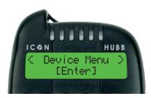
On activation of the bite Alarm the tone is replicated on the HUBB and the HUBB LED's replicate the alert colour shown on the bite Alarm. Depending on the HUBB's settings, the HUBB will also vibrate on alert.
