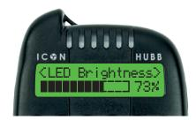
Go to **'LED Brightness'** to change the brightness of the LED's displayed on the bite Alarm.
