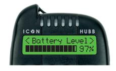
Navigate to the option 'Battery Level'. This provides a detailed measurement of the Alarms battery level.
