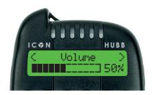
In 'Advanced Menu' go 'Alert Volume' to adjust the volume of the bite Alarm alert.
