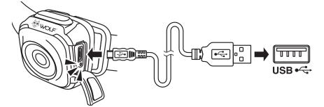
Inspect headlight for proper operation prior to using. Plug in the USB cable with battery source. The light will indicate charging status as follows:
